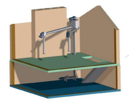
Two-level transport, with outlet into two boilers
